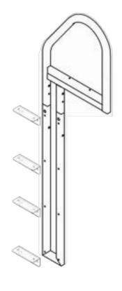
The Step Boards (C) will sleeve over the Step Bracket (D) and are fastened using two M6x20mm bolts/nuts (AA) on each side of the Step Board. Attach each Step Board to one of the Side Frame assemblies then position the second Side Frame assembly inside the Step Boards, tighten all bolts/nuts to complete assembly.
