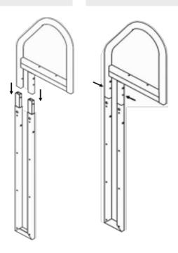
Mount the Step Brackets (D) to the Ladder Frame by aligning the pre-drilled holes and fastening with M6x40mm bolts/nuts (BB). Repeat for second side
