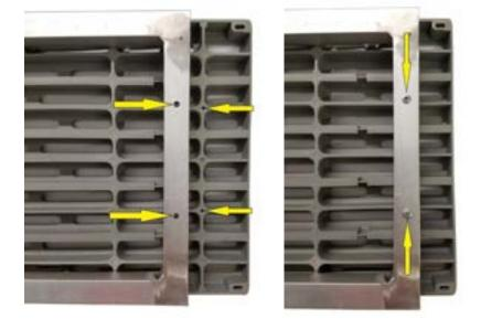
**Poly**: Align Aluminum Bench Frame (B) to pre-drilled holes on the bottom side of the Poly board using included M4x40mm Pan Head Screws (DD). Secure each Frame with (6) screws.
