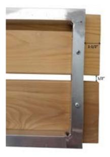
**Cedar**: Mount Aluminum Bench Frame (B), maintaining a 1/2" space between boards and a 1-1/2" space from the edge. using included M4x40mm Pan Head Screws (DD). Secure each Frame with (6) screws.
