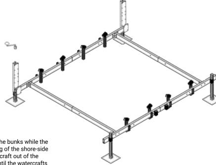
Operate the Boat Lift by guiding your watercrafts onto the bunks while the levelers are in the lowest position. Make sure the setting of the shore-side drop legs are high enough to keep the bow of the watercraft out of the water when resting on the lift. Then raise the levelers until the watercrafts are out of the water. Each leveler is operated independently, so raise or lower each leveler about 6" at a time.
